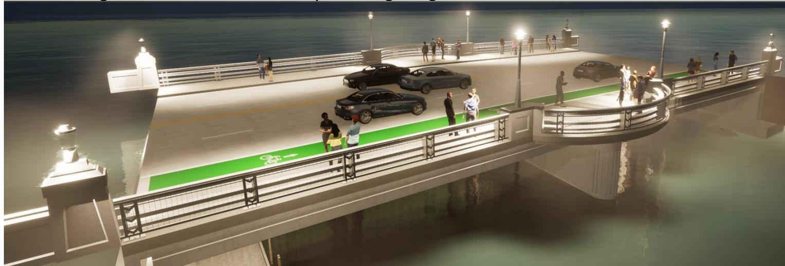
End Pylon Option 4 with Custom Luminaires and Forms+Surfaces LED Post-Top Luminaire on Mid-Bridge Pilasters and Under Top Rail Lighting
