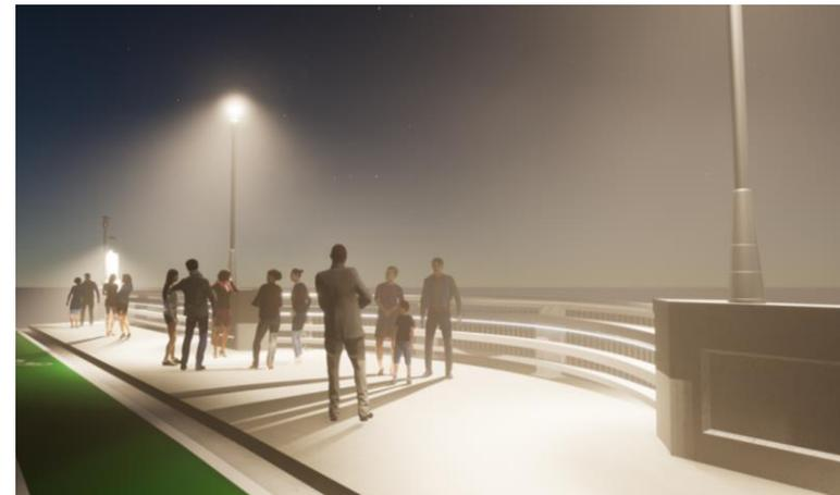
Bridge Rail Option 2 with Metal Vehicular Bridge Rail with Metal Pedestrian Fence, Forms+Surfaces LED Post-Top Luminaire on Mid-Bridge Pilasters and Under Top Rail Lighting
